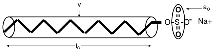
FIGURE 15.10. The geometric approach to the evaluation of surfactant aggregation processes is based on three molecular quantities: (a) the minimum interfacial area occupied by the head group, a_0 ; (b) the volume of the hydrophobic tail (or tails), v ; and (c) the maximum extended length of the tail(s) in a fluid environment, l_c .
